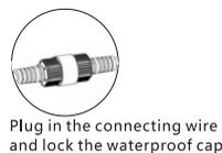
Plug in the connecting wire and lock the waterproof cap
